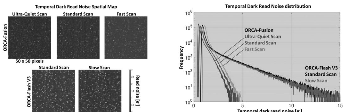
Figure 1: Spatial map and histogram comparison of temporal dark read noise between the next generation sCMOS camera (ORCA-Fusion) and the previous sCMOS camera (ORCA-Flash V3).
