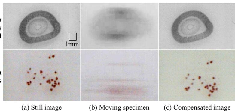
Figure 2: Comparison of result between still, moving, compensated images (after trimming and color correction)
