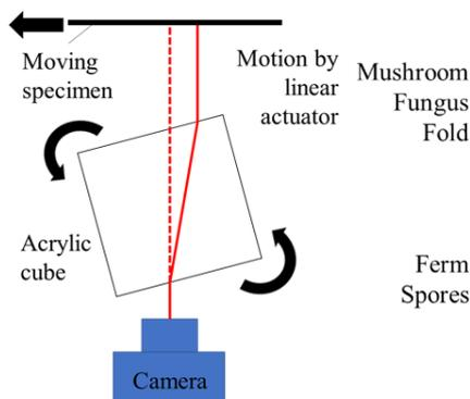
Figure 1: Schematic diagram of motion-blur compensation
