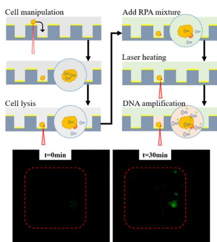
Figure 1. Cell trapping with a focused laser 785nm spot and the subsequent steps for cell lysis; Recombinase Polymerase Amplification (RPA) of target nucleic acids, as indicated by an increase in fluorescence signal at 30 minutes after laser heating by the laser spot (Single cell: Leukemia cancer cell)
