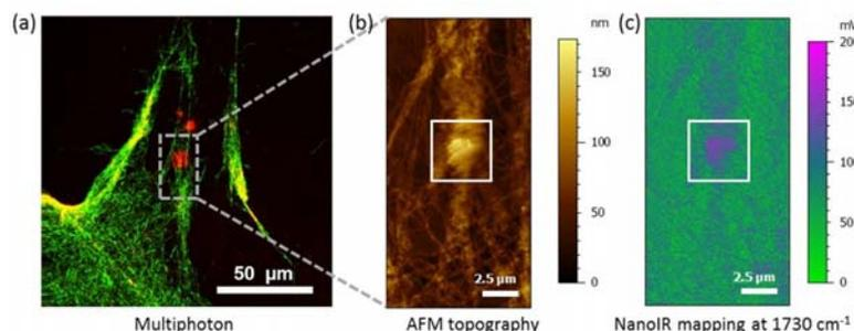
**Figure 1:** Correlative measurement of (a) multiphoton signals (2PEF in red color, SHG in green color), (b) AFM topography and (c) AFM-IR mapping at  $1730\ \text{cm}^{-1}$  after thermal denaturation of collagen fibrils with the AFM tip (white square).
