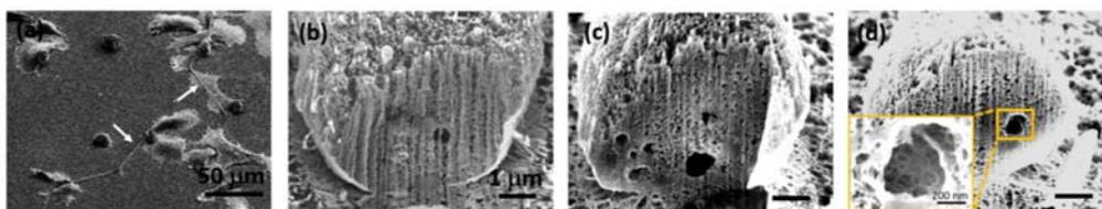
Figure 1. Images of SEM. Different cross sections of a TNT were revealed with FIB.
