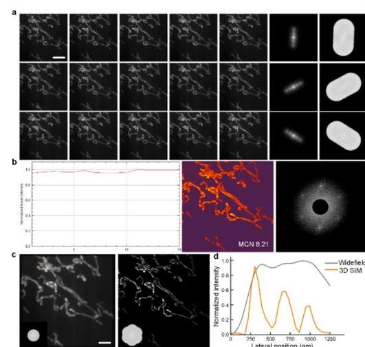
A 3D SIM image stack is presented in Fig. 1. Contrast to the widefield image, we can observe the hollow globular mitochondrial morphology, the intermediate mitochondrial structures, and the interconnected tubular network morphology with more details. The frequency distribution, modulation contrast, and channel intensity profile are also shown, illustrating the performance of our system.
