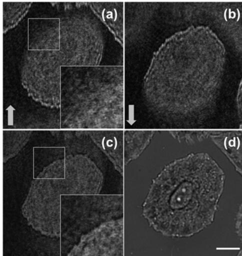
Figure 1: (a-b) Conventional and (c) switched surface plasmon microscopy images of a cell. (d) Bright-field image (scale bar: 10  $\mu\text{m}$ )
