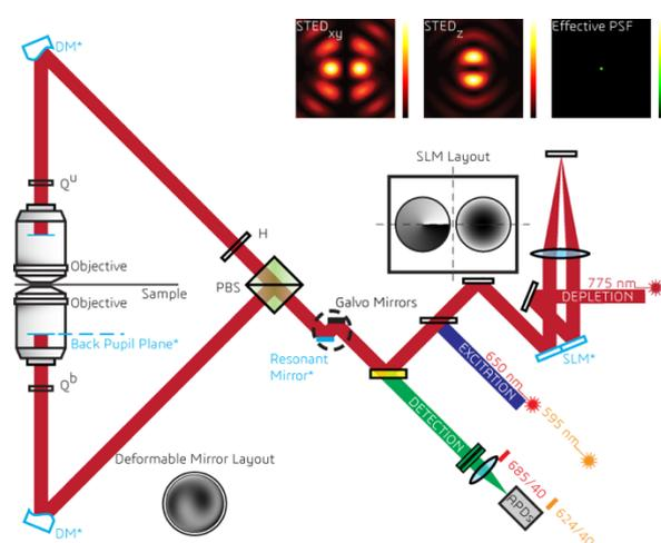
**Fig. 1** Simplified schematic of adaptive optical isoSTED nanoscopy.
