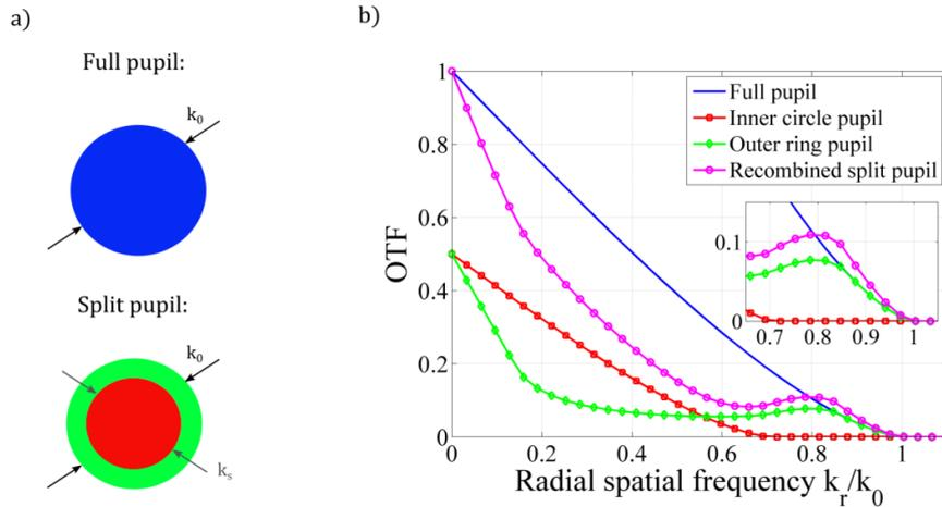
**Figure 1:** a) Visualization of circular full (blue) and split-pupil; split into an inner circle (red) and an outer ring (green). b) Efficiency-normalized OTF's corresponding to FP-, the two sub-pupils and the noise-normalized recombined result. ( $k_r$ : radial spatial frequency,  $k_0$ : system's cut-off frequency,  $k_s$ : being the split frequency).
