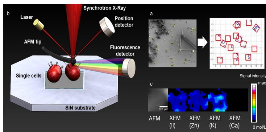
Figure 1. Schematics showing the experimental procedures initiated with (a) feature recognition and proposed planning scheme of target cells, followed by (b) XFM quantification and AFM topological measurement on single cells and (c) post-processing to derive the high resolution correlative images on one single bacterial cell (*Acinetobacter baumannii*).
