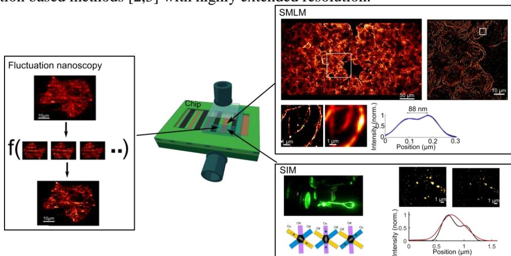
Fig. 1: Chip-based multi-modality TIRF nanoscopy: Fluctuation nanoscopy utilize intrinsic intensity fluctuations to generate a stack of images and an algorithm to extract a super-resolved image. Chip based *d*STORM generate super-resolved images over large fields of view. The photonic chip also supports SIM that harness standing waves generated by interfering waveguide structures.
