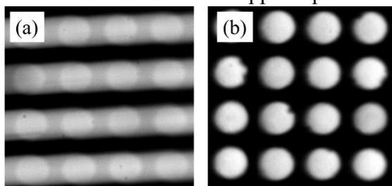
Figure 1: Motion-blur compensation during motion at a speed of 20mm/s
