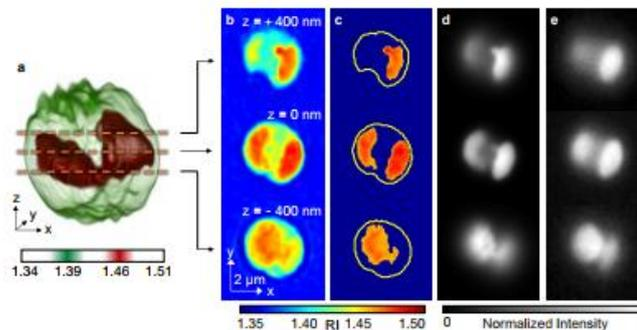
Figure 1: Identification of the lipid droplets inside an *N. oculata* cell: (a) A 3D rendered isosurface of RI distribution of the cell. (b) Cross-sectional images of different axial planes. (c) The identified lipid regions based on the RI threshold  $n > 1.46$ . (d) The emulated images generated from the RI. (e) The fluorescence images of the same cell stained with Nile red dye.
