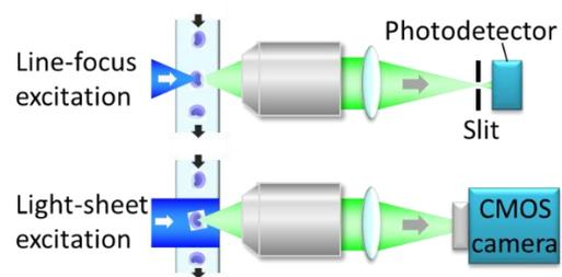
Fig. 1: Schematics of the confocal FIFC (top) and the light-sheet FIFC (bottom).
