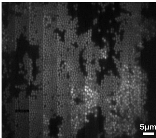
**Fig. 1:** Raman image of 1 $\mu\text{m}$  polystyrene beads, measured with the illumination of 11 lines and constructed with 3055 $\text{cm}^{-1}$ .
