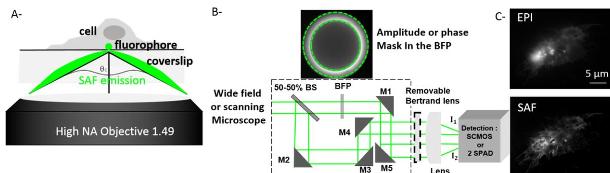
Fig. 1: A- Principle of SAF emission, B- dual imaging path for SAF detection C- Simultaneous images of CB1R receptor in HEK cells
