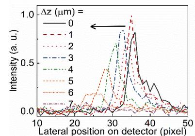
Fig. 1. Measured intensity profiles of an Airy beam emitted from a fluorescent bead at different axial positions ( $\Delta z$ ).
