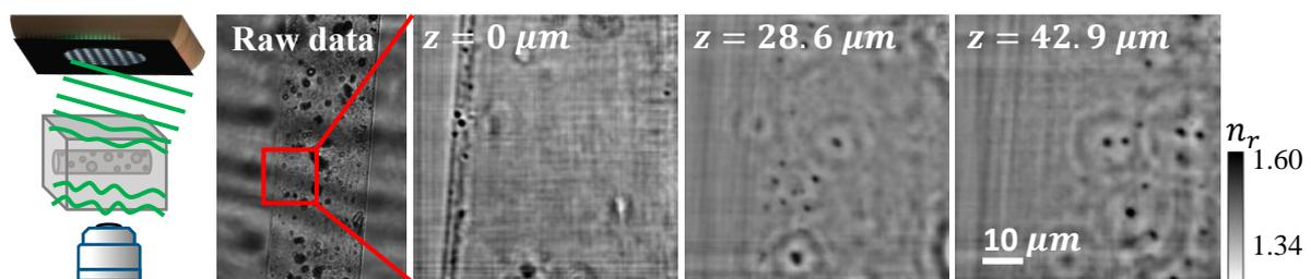
Figure 1: Reconstructed refractive index of a bead-filled lumen embedded in agarose.
