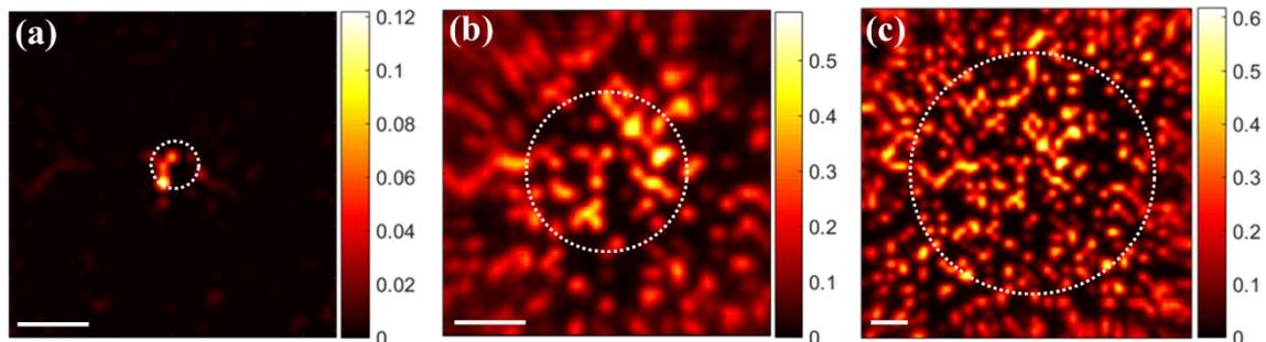
Figure 1: Comparison of imaging of fluorescent beads (7.8  $\mu\text{m}$  diameter) through random phase mask ( $\mu_s L=3.98$ ) (a) with pupil AO, (b) with CAOSG and (c) with CAOMG. The dotted circles are intended to determine the corrected FOV. Scale bar 25  $\mu\text{m}$ .
