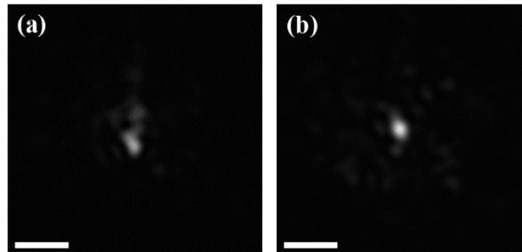
Figure 2: The focus before and after wavefront correction. (a) The distorted focus due to scattering effect introduced by a ground glass diffuser. (b) The recovered focus after wavefront correction. Scale bar 100  $\mu\text{m}$ .
