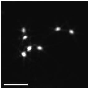
Figure 1: Seven focuses generated by pupil segment methods. Scale bar 300  $\mu\text{m}$ .
