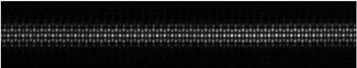
Figure 1: Example of a hexagonal lattice light-sheet pattern as observed in transmission.
