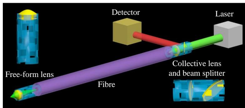
Figure 1: Schematic of an ultra-lightweight fibre-optical endoscope
