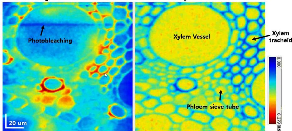
Fig. Real-time fluorescence lifetime imaging of maize vascular tissue based on the analog mean-delay (AMD) method (a) fluorescence intensity image (b) fluorescence lifetime image
