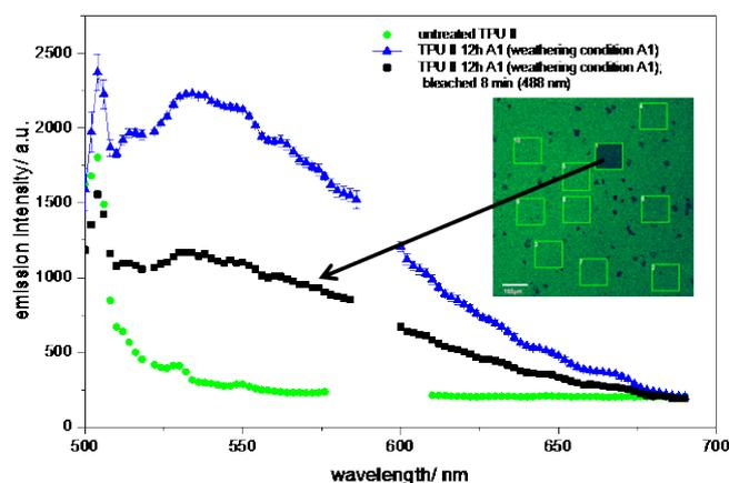
Fig. 1: Microscopic and spatially resolved fluorescence spectroscopic monitoring of accelerated aging of a TPU polymer.
