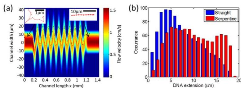
Fig1. (a) Flow velocity profile on a serpentine channel with a simulation of DNA dynamics. Insets show the shape of DNA before and after the channel. (b) Extension distribution of single  $\lambda$ -DNA molecules after 1.4 mm straight and serpentine channels (1000 simulations each).
