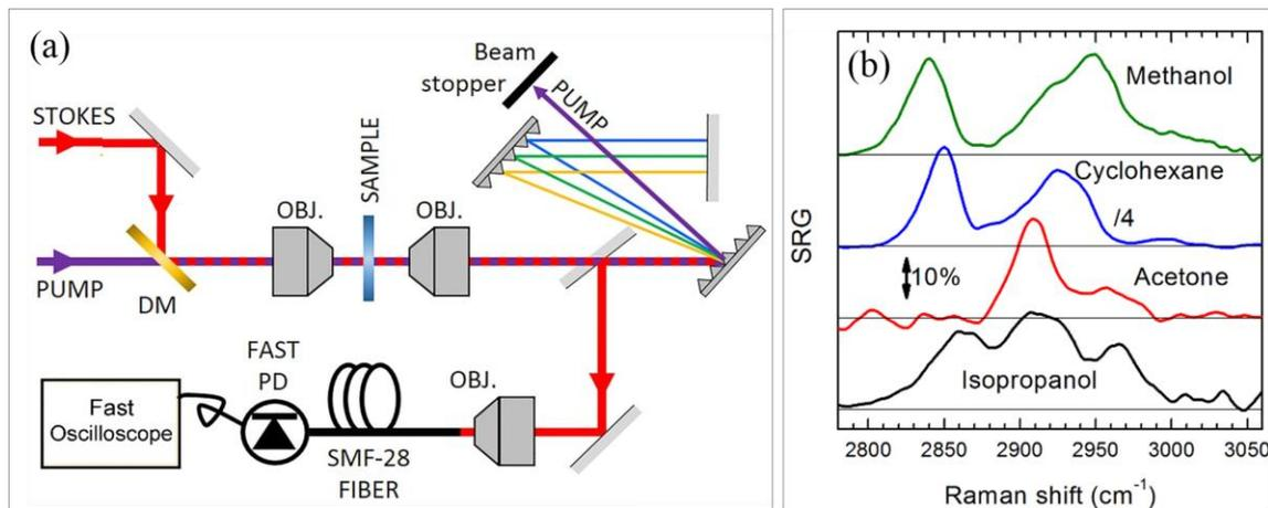
**Fig. 1:** (a) Schematic setup of the PTS-SRS. DM: Dichroic mirror, PD: photodiode. (b) SRS spectra of different solvents, averaged over 8 consecutive pulses (100  $\mu$ s acquisition time). Pump energy was 200 nJ on the sample. The cyclohexane signal has been divided by 4 for comparison.
