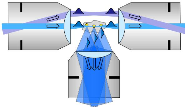
Figure 1: Schematic of the illumination and reference beams.
