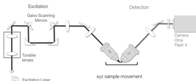
Principle setup of light sheet microscope
