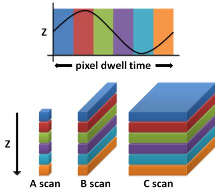
Fig 1: Simultaneous capture of multiple focal planes in A, B and C scans.
