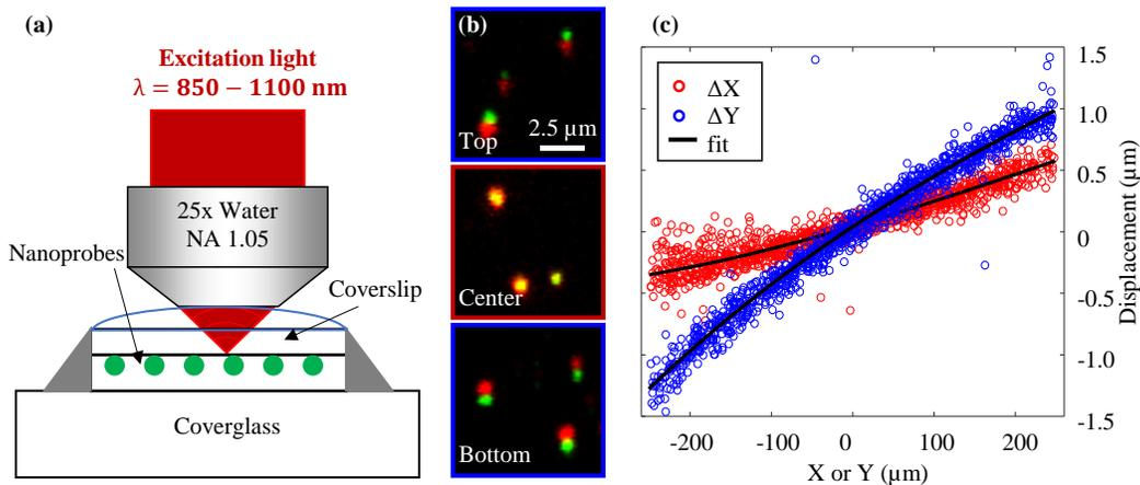
Figure: Quantification of lateral chromatic aberrations. (a,b) Nanoprobe are imaged at different excitation wavelengths (for e.g.  $\lambda = 850$  &  $1100$  nm, green and red signal in (b), respectively). (c) Lateral chromatic aberrations are estimated across the field of view by comparing the positions of each nanoprobe imaged at different excitation wavelengths (for e.g.  $\lambda = 850$  &  $1100$  nm).
