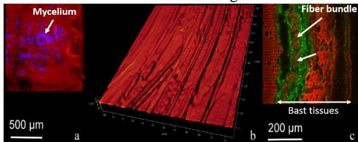
Figure 1 : Autofluorescence pictures at 408 nm, 480-540 nm emission and 638 nm excitation, 650-750 emission (a) retted hemp stem surface – (b) 3D reconstruction of unretted hemp stem surface – (c) retted hemp stem section
