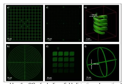
We have developed a new process that enables the etching of long-term stable fluorescent patterns (cf. figure on the left) with sub-micrometer sizes in 2D and 3D inside glass. Based this new process, fluorescent patterns and dedicated image analysis algorithms are shown to be suitable for complete and quick OC of fluorescence microscopes [6]. Nonexhaustively, this new solution
