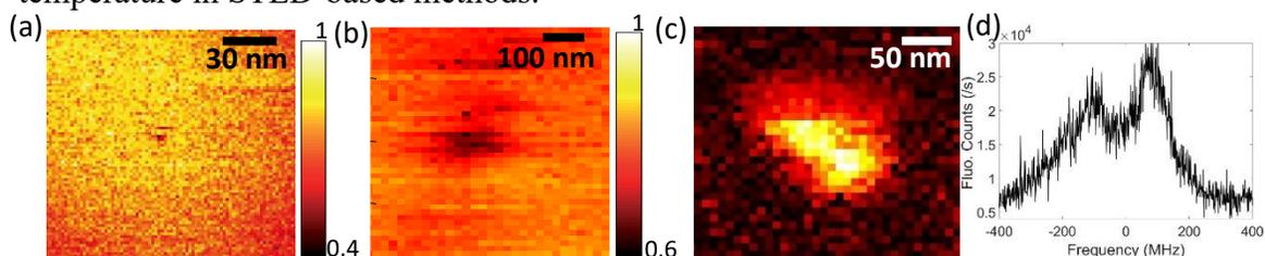
Fig.1 (a) ESSat image of a single DBATT molecule in Octadecane matrix in the (a) lateral plane (XY) using doughnut beam and (b) axial plane (XZ) using  $0/\pi$  beam (c) resolving two molecules with overlapping resonances and (d) fluorescence excitation spectrum. Color-bar giving the relative fluorescence intensity.
