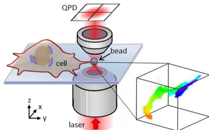
Figure 2: Schematic of microscope setup
