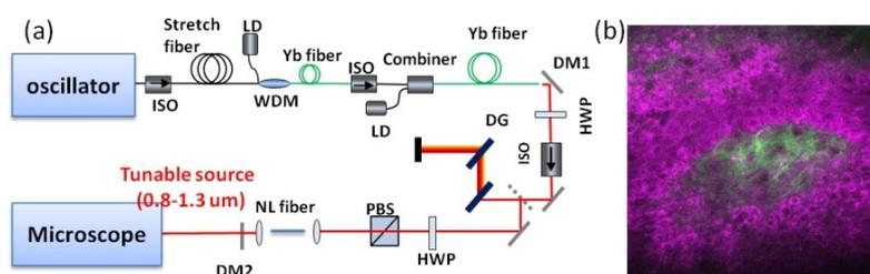
Fig. 1. (a) Schematic of novel fiber-sources based on Yb-fiber oscillators with various repetition rates. DM: dichroic mirror, ISO: isolator, LD: laser diode, DG: diffraction grating, NL fiber: nonlinear fiber, HWP: half-wave plate, PBS: polarization beam splitter. (b) Harmonics imaging of *ex vivo* human skin using 1200nm femtosecond pulses with 50MHz repetition rate. Magenta: THG; Green: SHG; Imaging size: 200 $\mu$ m  $\times$  200 $\mu$ m
