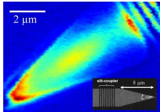
Fig. 1: Reflectance-variation image of a taper by a raster-scanned probe beam @532nm  $\approx$ 1ps after the plasmon excitation by a pump beam @800nm (fixed on the coupler).
