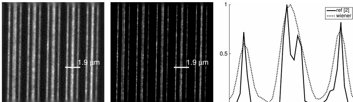
Figure 1: Reconstruction of the Argolight test pattern L from a series of 100 speckle illuminations: (left) Deconvolution of the mean of the dataset; (center) Blind-SIM reconstruction; (right) Line section plot extracted from both reconstructions.
