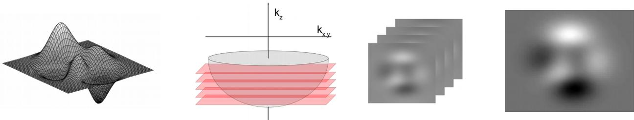
From left to right. 3-D surface to be reconstructed. Reflection OTF sliced along  $k_z$  axis. Ensemble of intermediary reconstructed surfaces obtained by inverse FFT of each slice. Reconstructed final surface as a combination.
