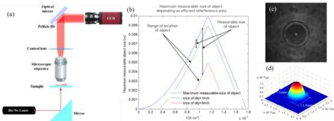
Figure 1: (a) Optical setup of the proposed SA-OAI system, (b) Maximum measurable-size of the object depending on the effective interference area (EIA), (c) Recorded holographic interference pattern, and (d) Reconstructed 3-D shape of the object
