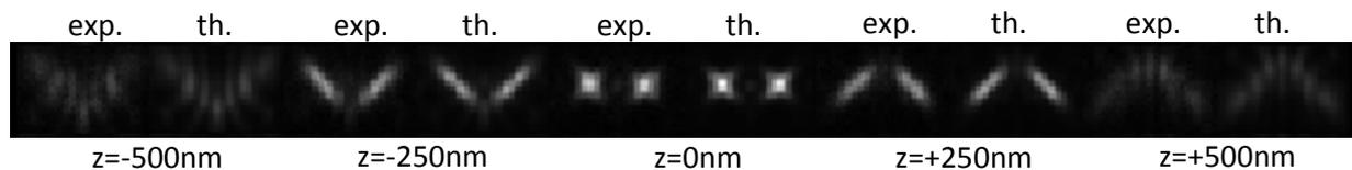
*Through-focus images of the double astigmatic engineered PSF measured with our adaptive optics aberration corrected microscope on green 175 nm diameter beads and corresponding fits with the vectorial PSF model, showing excellent correspondence.*
