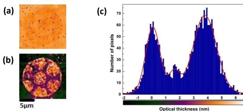
Figure 1: (a) Intensity and (b) phase shift images of structured graphene layers deposited on glass substrate. (c) Histogram plot of the phase shift image.
