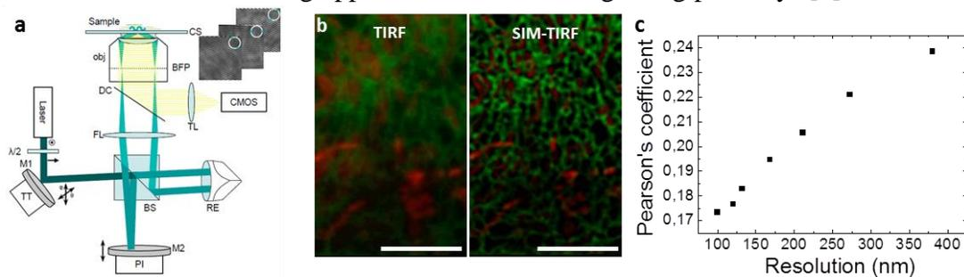
**Fig. 1:** (a) High resolution TIRF-SIM microscope schema. (b) Dual color images of ER (in green) and mitochondria (in red) taken in TIRF (left) and in TIRF-SIM (right). Scale bar: 1  $\mu\text{m}$ . (c) Pearson's colocalization coefficient as a function of the images spatial resolution.
