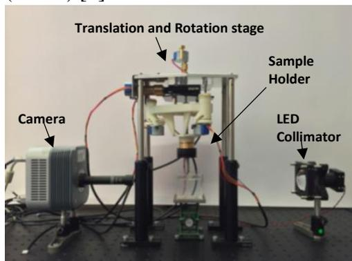
Figure 1: Picture of the current OPT set-up. An Andor CLARA camera is placed on the far left, the 3D-printed motion stage and sample holder in the center, and the transmission illumination system on the right.
