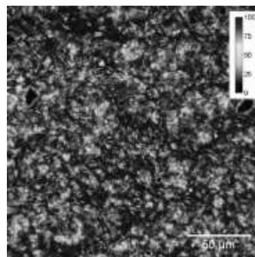
Figure 1: Raman MCR concentration map of solid fat in a dispersion of 20% solid fat (MFC) in sunflower oil.
