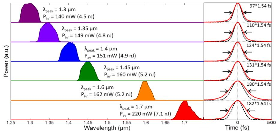
Fig. 1. Er-fiber laser based, widely tunable femtosecond source. Left column: typical optical spectra labeled with peak wavelength, average power, and pulse energy. Right column: corresponding autocorrelation traces showing that the resulting pulses are 100-200 fs in duration.
