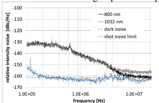
Fig.1 RIN measurement of the light source
