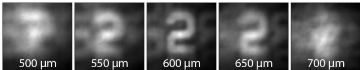
Figure 1. Demonstration of optical sectioning in the widefield configuration (effective focal distance of the imaging system is given for each image).
