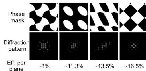
**Figure 1:** Different diffraction masks designs for multifocus microscopy allowing a flexible number of imaging planes and exhibiting multicolor properties.
