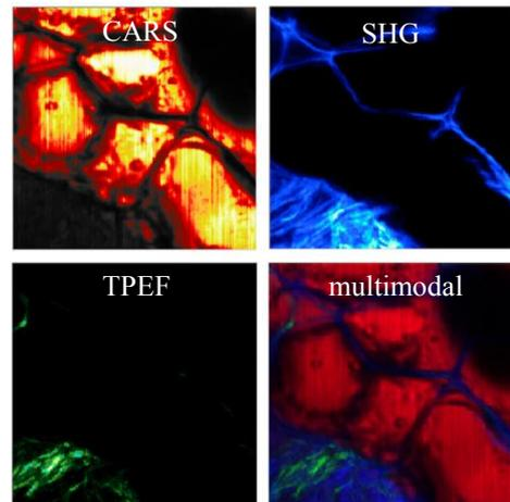
Fig. 2: With a spectral focusing phase function simultaneously measured signals from human skin tissue.
