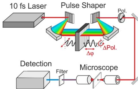
Fig. 1: Experimental setup for single-beam multimodal microscopy.
