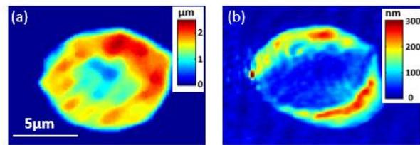
Figure 2: Quantifying the membrane fluctuations of a live RBC
