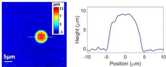
Figure 1: Quantitative phase imaging of polystyrene bead
